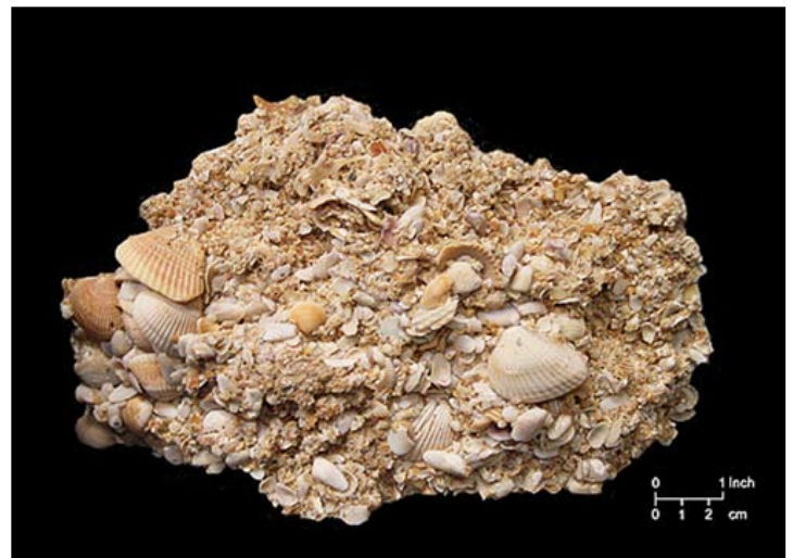
Anastasia Formation. This is an example of a very high shell concentration lime rock, found along much of the Southwest Florida Coast. Courtesy Florida Geological Survey.
