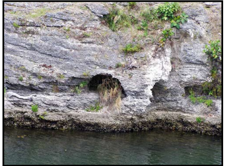
Collier County Main Canal. Top layer of humus and silica sand supports dense foliage. Lower layer blends from nearly pure calcite limestone to mixed shells and oolite.
