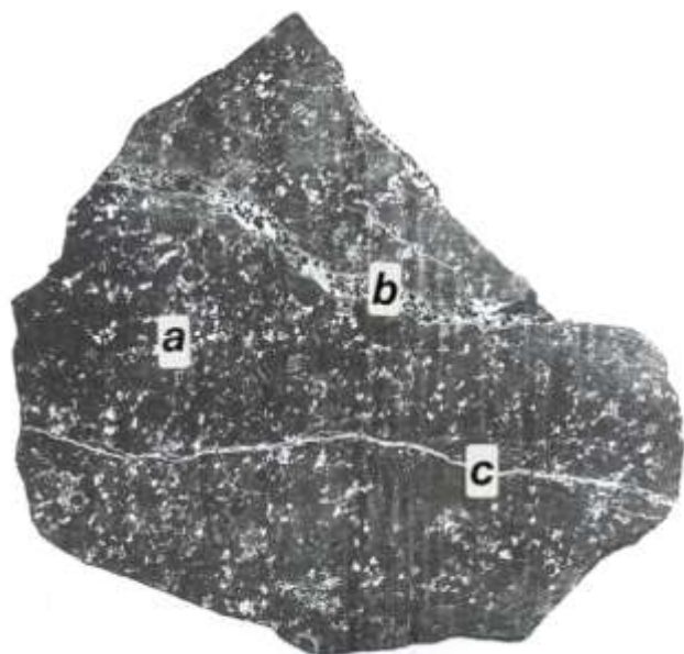
composition can be seen A) in the numerous inclusions; B), a darkly speckled intrusionary layer; and C) what appears to be a fracture line running across the section. Photograph courtesy of the Smithsonian Institution, Washington, DC. Scale line unavailable.
